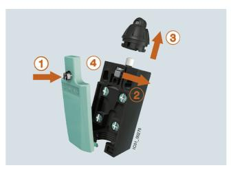
Open the cover (1) Actuate the locking lever (2) Replace the head (turnable by 16 x 22.5°) (3) Lock and close the cover (4)
