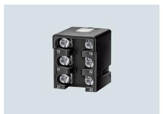
The 3-pole contact block with snap-action or slow-action contacts is regularly available for all enclosure forms. The same installation space is required as for a 2-pole block. The version with 1 NO + 2 NC offers, for example, more safety through redundant shutdowns (2 NC contacts) with simultaneous signaling (NO contact). The 3-pole blocks are also available with make-before-break and with 2 NO + 1 NC.
